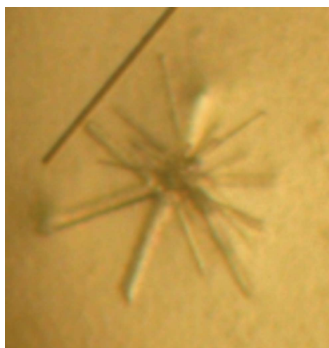
Figure 2 Crystals of CtXyl5A obtained by hanging-drop vapour diffusion in the presence of 40% (v/v) 2-methyl-2,4-pentanediol and 10–20% 2-propanol. The largest crystals in the needle clusters are approximately 200 \times 10 \times 10 \mu\text{m} in size.
